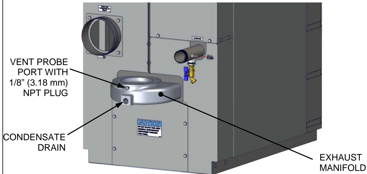
Figure 4-2. Analyzer Probe Hole Location
