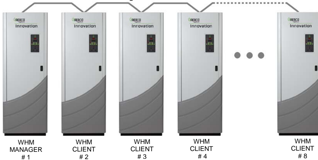
Figure 8-3. Typical Daisy-Chain Modbus/RS485 Network
