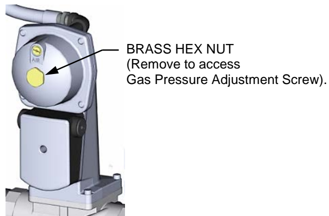
Figure 4-3: Gas Pressure Adjustment Screw Location
