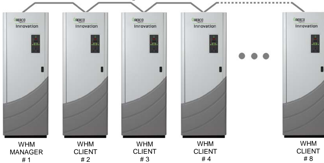
Figure 8-3. Typical Daisy-Chain Modbus/RS485 Network
