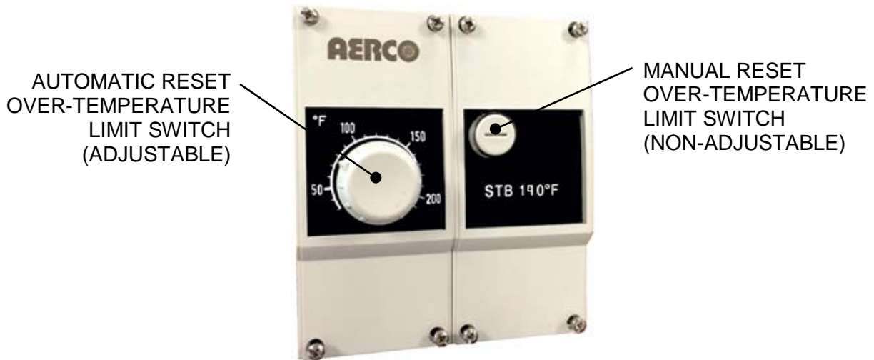
Figure 5-2. Over-Temperature Limit Switch Setting
