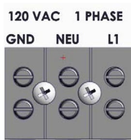
Figure 2-10. AC Terminal Block Configurations
